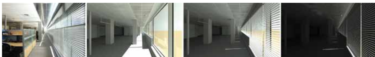
Figure 5. Excerpts from the pattern sequence showing the as-built condition (far left) and daylight renderings of the space with blinds retracted under a sunny sky, with light redirecting blinds deployed under a sunny sky, and with the same blind position under an overcast sky (far right).
