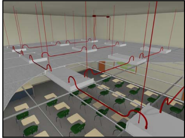
Figure 15 – Typical Recessed Classroom (Ceiling grid supports omitted)
